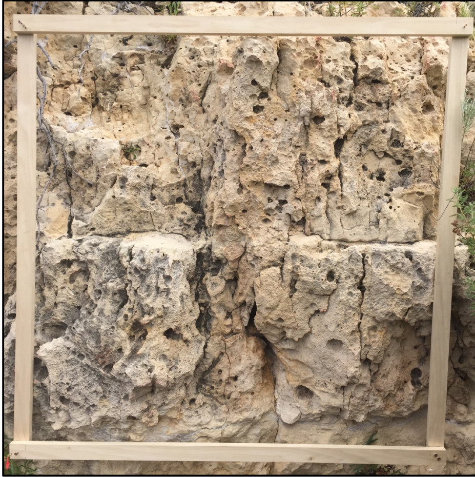
Figure 7: Wooden tool measuring 1 m 2 constructed for fracture analysis, pictured against an outcrop of Kaibab Limestone. All fractures within the square were measured.
