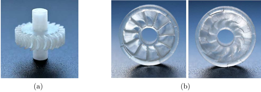
Figure 4.8: Physical model of turbine components: (a) rotor and (b) stator inlet (left) and outlet (right).
