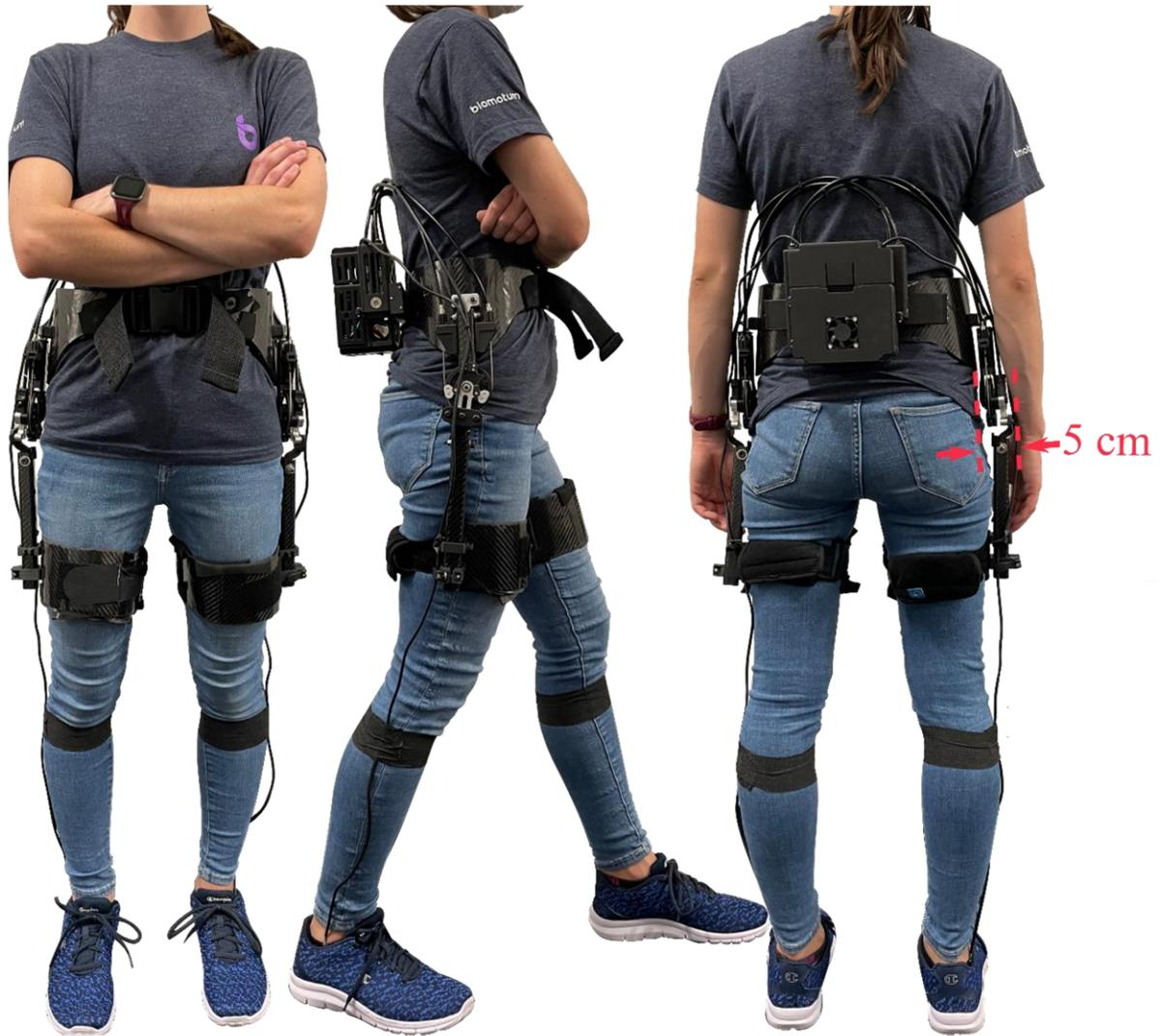
*Figure 14 . Pictures of our hip exoskeleton.*
