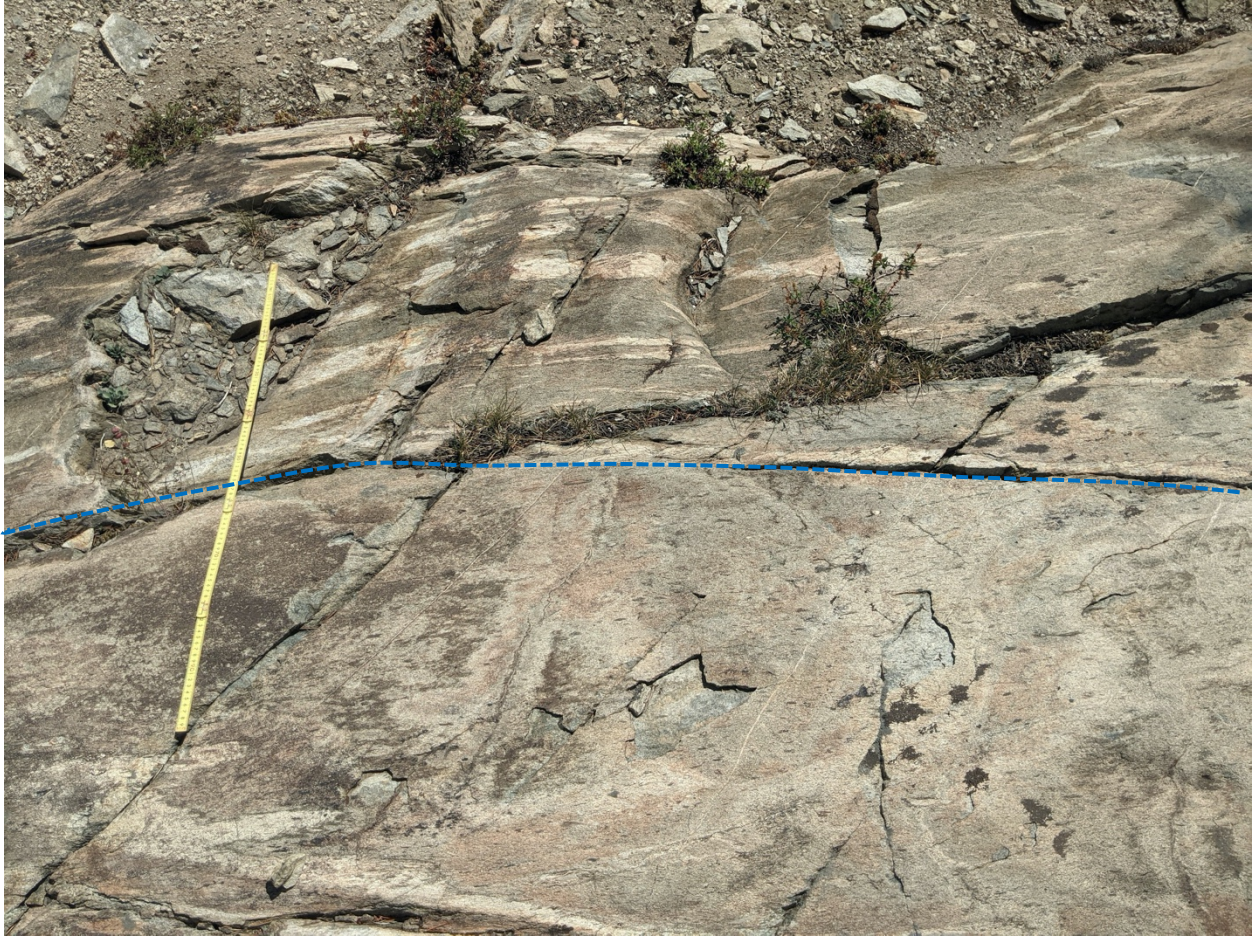
Figure 18: Contact (blue dashed line) between pumice conglomerate (top) and upper grey lithic tuff (bottom). Note how sparse the clasts are at the contact. Ruler is 1 m long.
