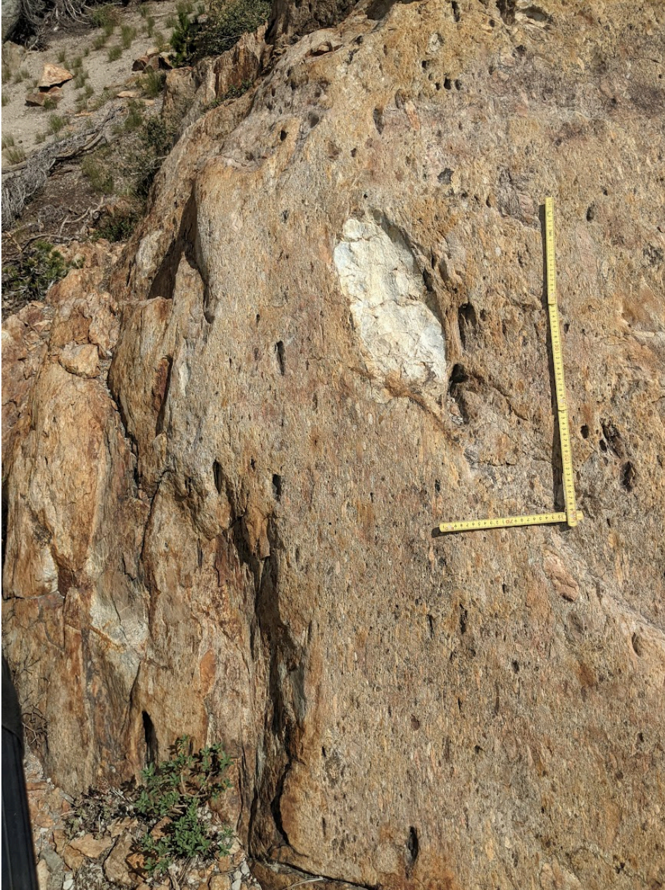
Figure 24: Quartzite conglomerate with a variety of clast types, shapes, and sizes, with many void spaces. Dark oval shapes are voids and the large white clast is quartzite. Black ruler increments are 1 cm.
