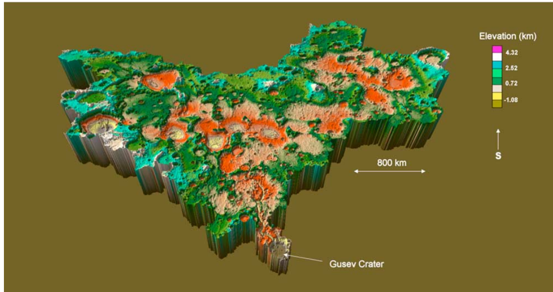
Figure 2. Ma'adim Vallis watershed as reconstructed using the MOLA data. Its size is comparable to the largest terrestrial watersheds (e.g., Amazon basin). A series of basins connect to the main hydrographic system, which empties in Gusev. The topography and morphology seem to indicate that they were a series of closed basins rather than a giant one and that ice/snow played a substantial role in their activation.
