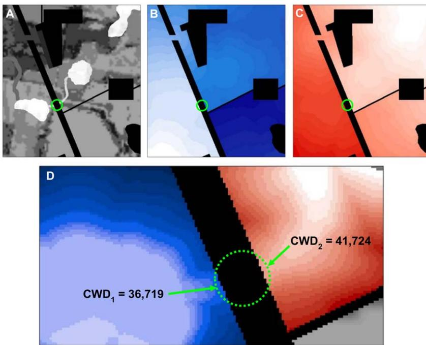
**Figure 2. Detail of resistance and *CWD* surfaces with circular moving window.** For a window with a diameter of 60 m (20 pixels) centered on the barrier, the arrows show the pixels in the window that have the lowest *CWD* to each patch (values shown are in weighted meters). Because the lowest *CWD* values from each patch will always be found on the edge of a moving window, only pixels on the perimeter need to be examined, increasing processing efficiency. doi:10.1371/journal.pone.0052604.g002
