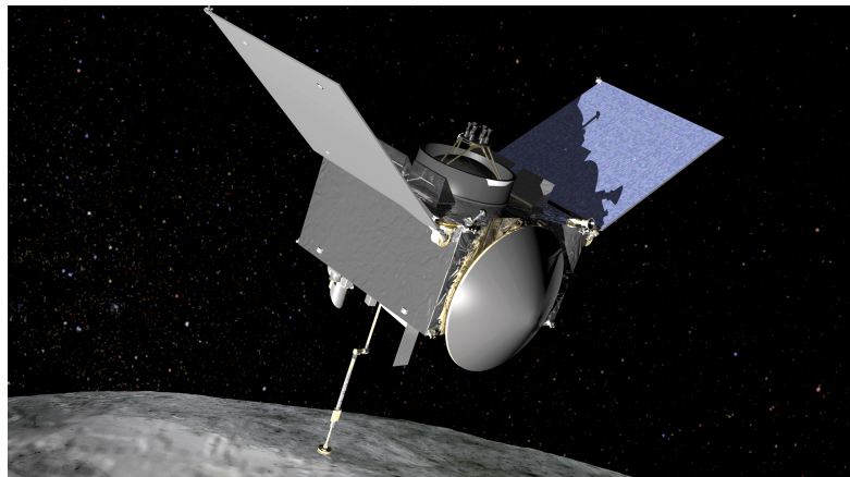
Figure 34. An animation of OSIRIS-REx with the TAGSAM extending from the bottom.
