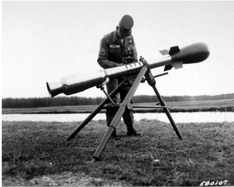
Figure 13. A Davy Crockett “tactical” nuclear weapon system being tested in 1961.
