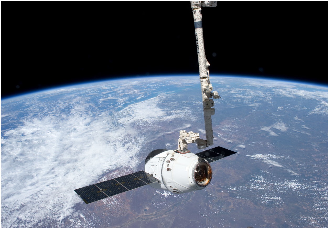
Figure 16. The SpaceX Dragon commercial cargo craft—grappled by the Canadarm2—became the first commercially developed space vehicle to be launched to the International Space Station. It was successfully berthed to the Harmony node at 12:02pm on May 25, 2012.
