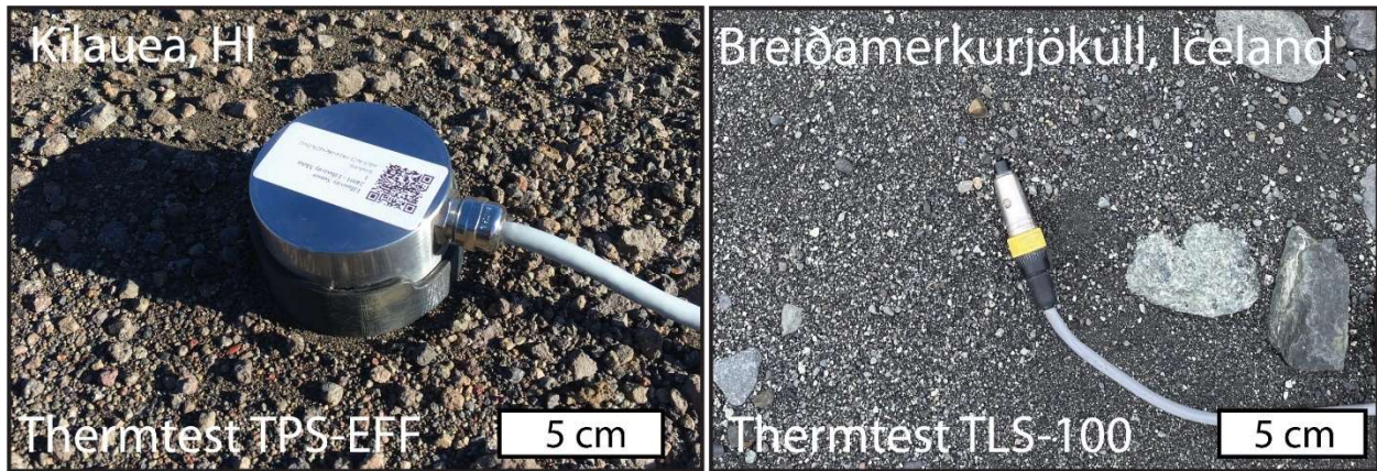
Figure 4-2. Thermtest probes collecting thermophysical data in the field. Poor contact due to surface roughness or porous soil had to be mitigated.
