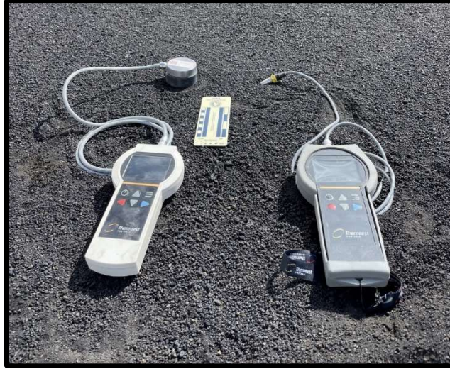
Figure 3-9. Thermtest TPS-EFF (left) and TLS-100 (right) capturing thermophysical data at Woodhouse Mesa for model validation.
