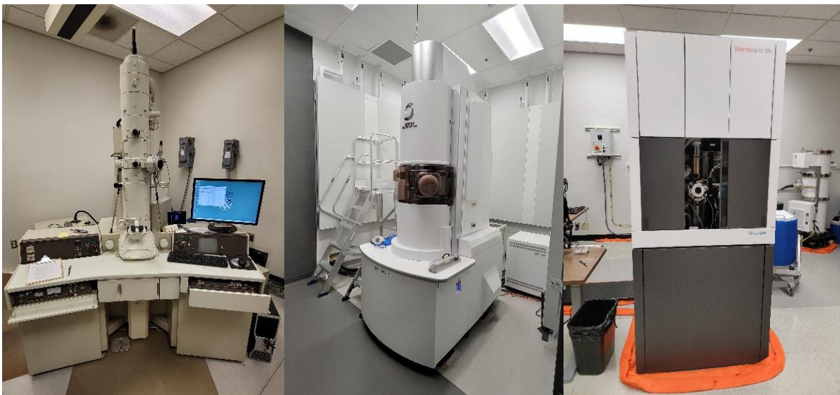
Figure 2-2: Images of different types of transmission electron microscopes. From left to right: JEOL Jem, JEOL NEOARM, Talos F200i. The JEOL Jem uses a heated filament type gun and is controlled at the microscope. Both the newer NEOARM and F200i use cold field emission guns and are controlled remotely.
