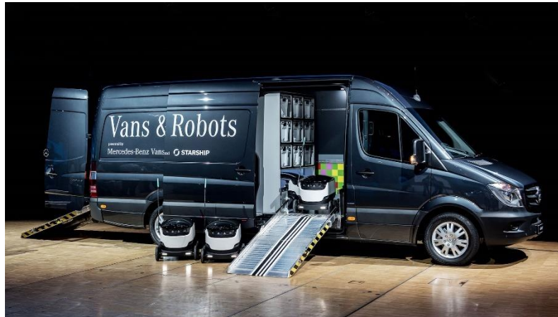
Figure 4: Example of a mothership and SADR combined delivery
