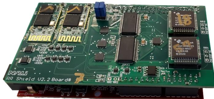
**Figure 5.1:** Chipkit Wi-Fire mounted with custom PCB used for analog key encapsulation
