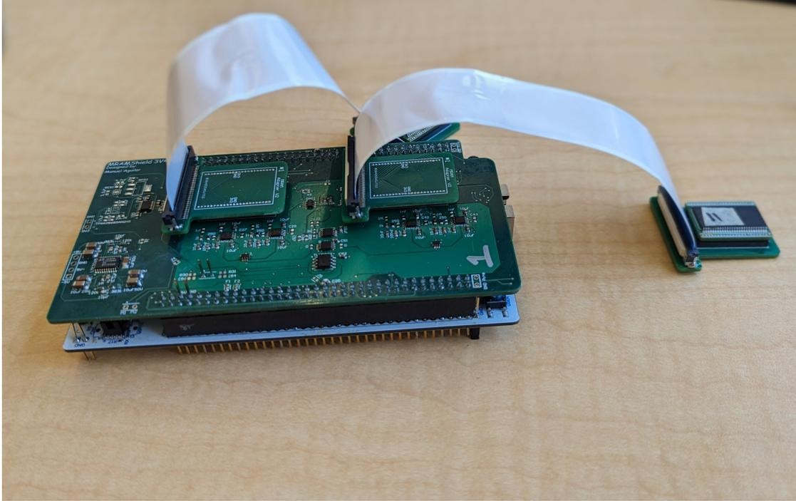
**Figure 4.3:** MRAM Adapter with Flat Flex Cable, used to isolate the MRAM device from external circuitry during temperature testing
