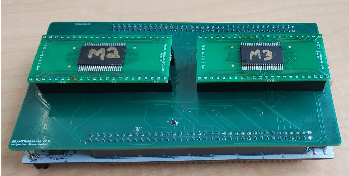
**Figure 3.3:** Nucleo-144 Developer Kit, Custom PCB, and SRAM Devices
