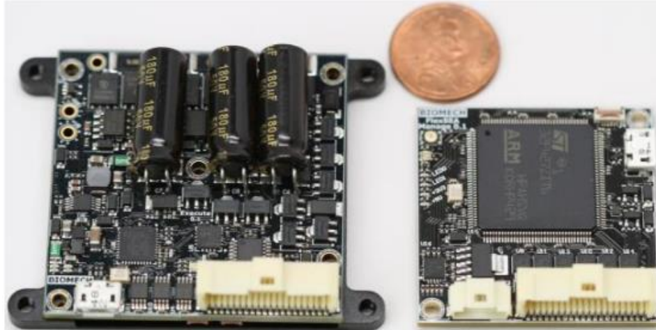
Figure 2: FlexSEA Printed Circuit Board [5]. A modular design for wearable robotics composed of high-level computation modules and low-level sensing and actuation modules.
