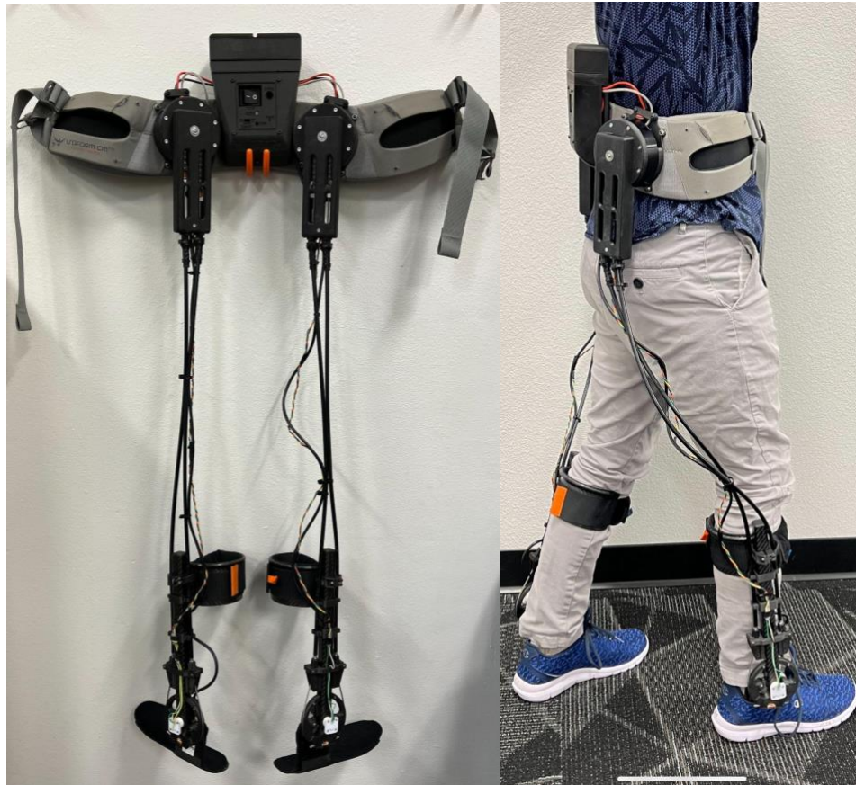
Figure 5: High Power cable-driven ankle exoskeleton constructed using the modular platform for wearable robotics.
