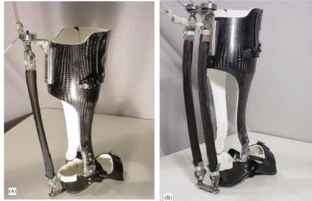
Figure 26: Artificial pneumatic muscle powered ankle exoskeleton. (a) single muscle, (b) dual parallel muscle [70]
