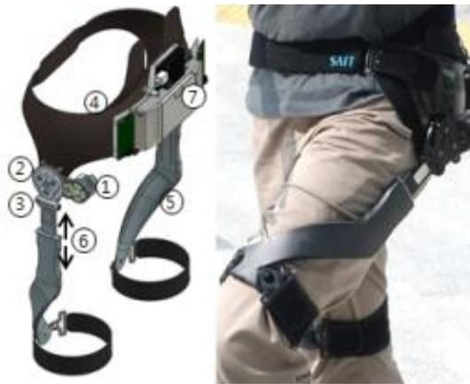
Figure 6: Samsung Institute of Technology Hip Exoskeleton. 1) BLDC Motor, 2) joint actuator, 3) passive hinge for abduction/adduction, 4) hip brace, 5) thigh frame, 6) spring loaded sliding mechanism, 7) CPU and battery [39]
