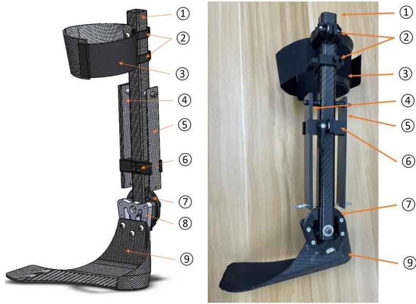
Figure 29: Final AFO Design. (1) upright, (2) cuff sliders with tightening cam mechanisms, (3) calf cuff, (4) plantarflexion assist leaf spring, (5) dorsiflexion assist leaf spring, (6) upright slider with tightening cam mechanism, (7) ankle pulley, (8) pulley-to-footplate adapter, (9) footplate
