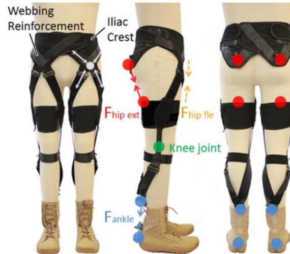
Figure 13: Ankle-Hip Soft Exosuit. Anchor joint anchor points (blue), hip joint anchor points (red) [49]
